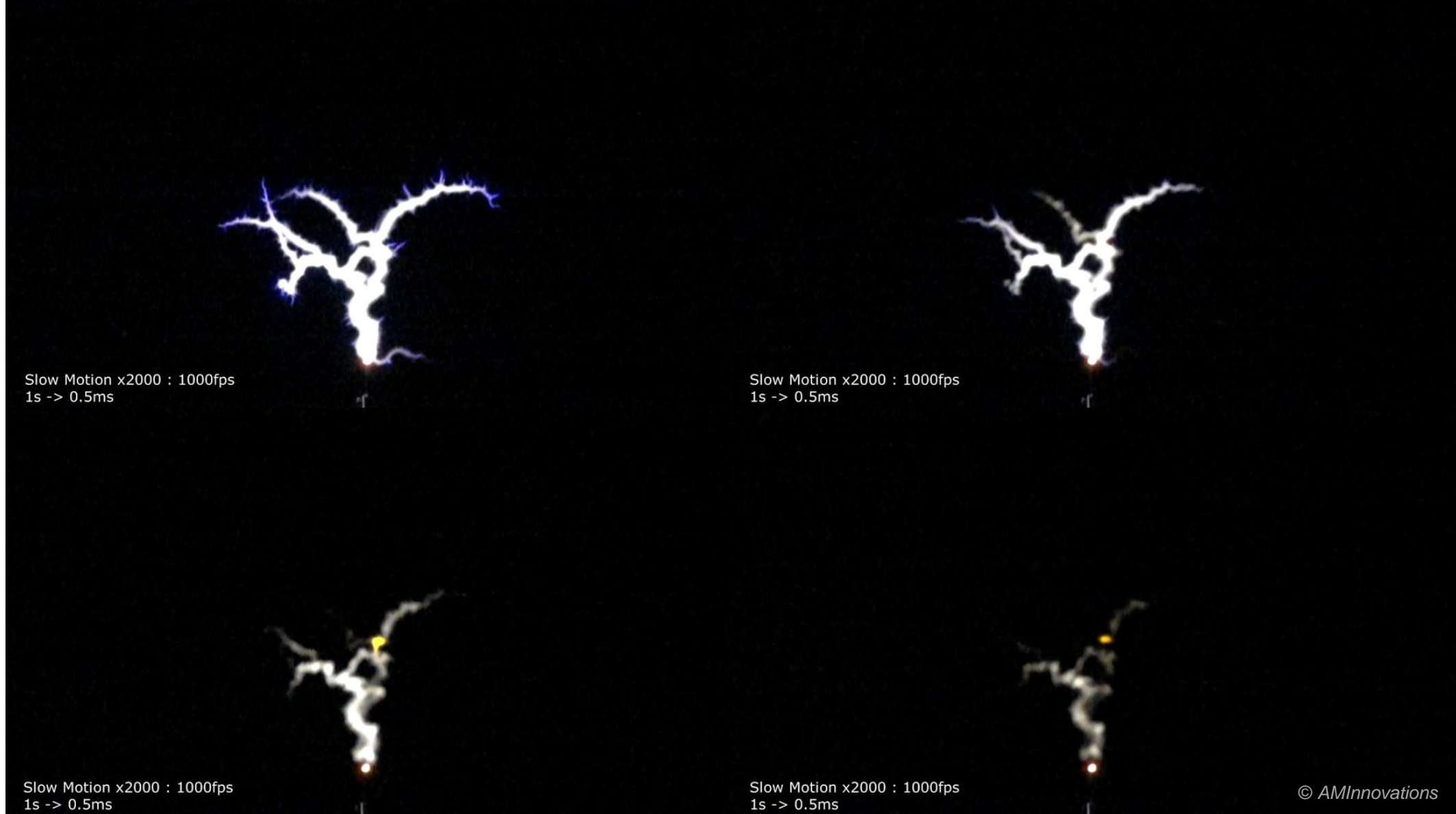
Slow motion from Sony RX10M2 1000fps – Extinguish of discharge over 4 frames (4ms)
