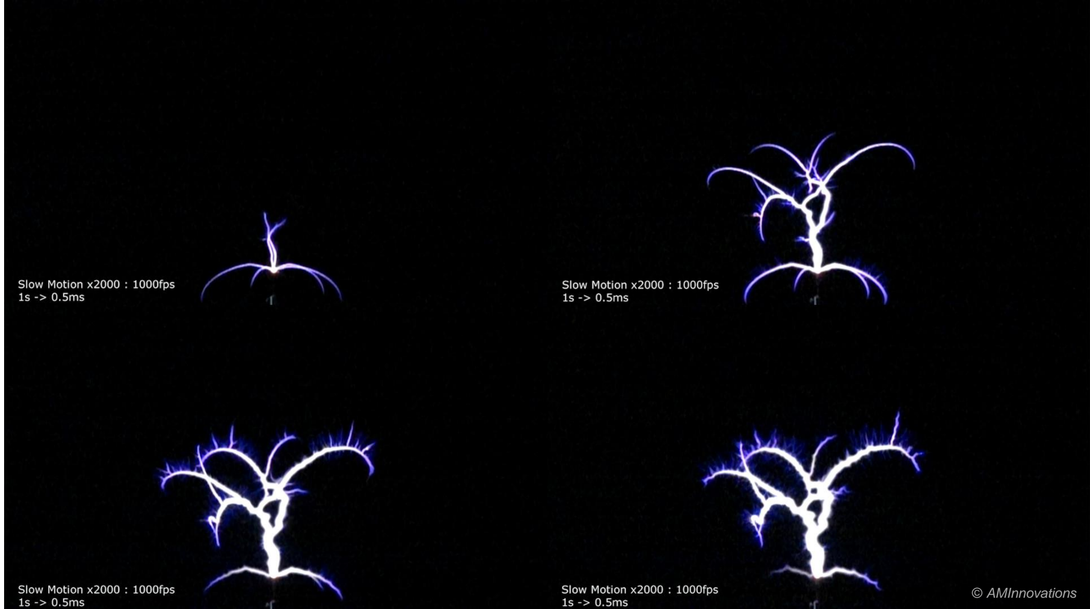
Slow motion from Sony RX10M2 1000fps – Growth of discharge over 4 frames (4ms)
