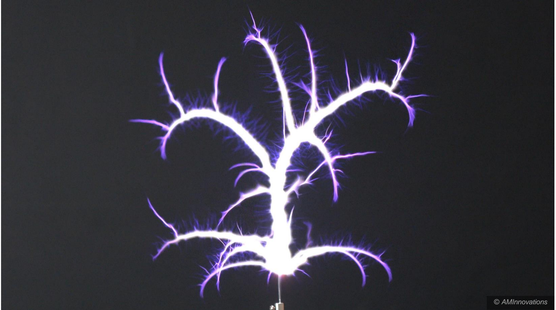
4K Images taken by the Sony RX10M2 - Micro-filaments (blue hedge) that appear to result from parasitic oscillation
