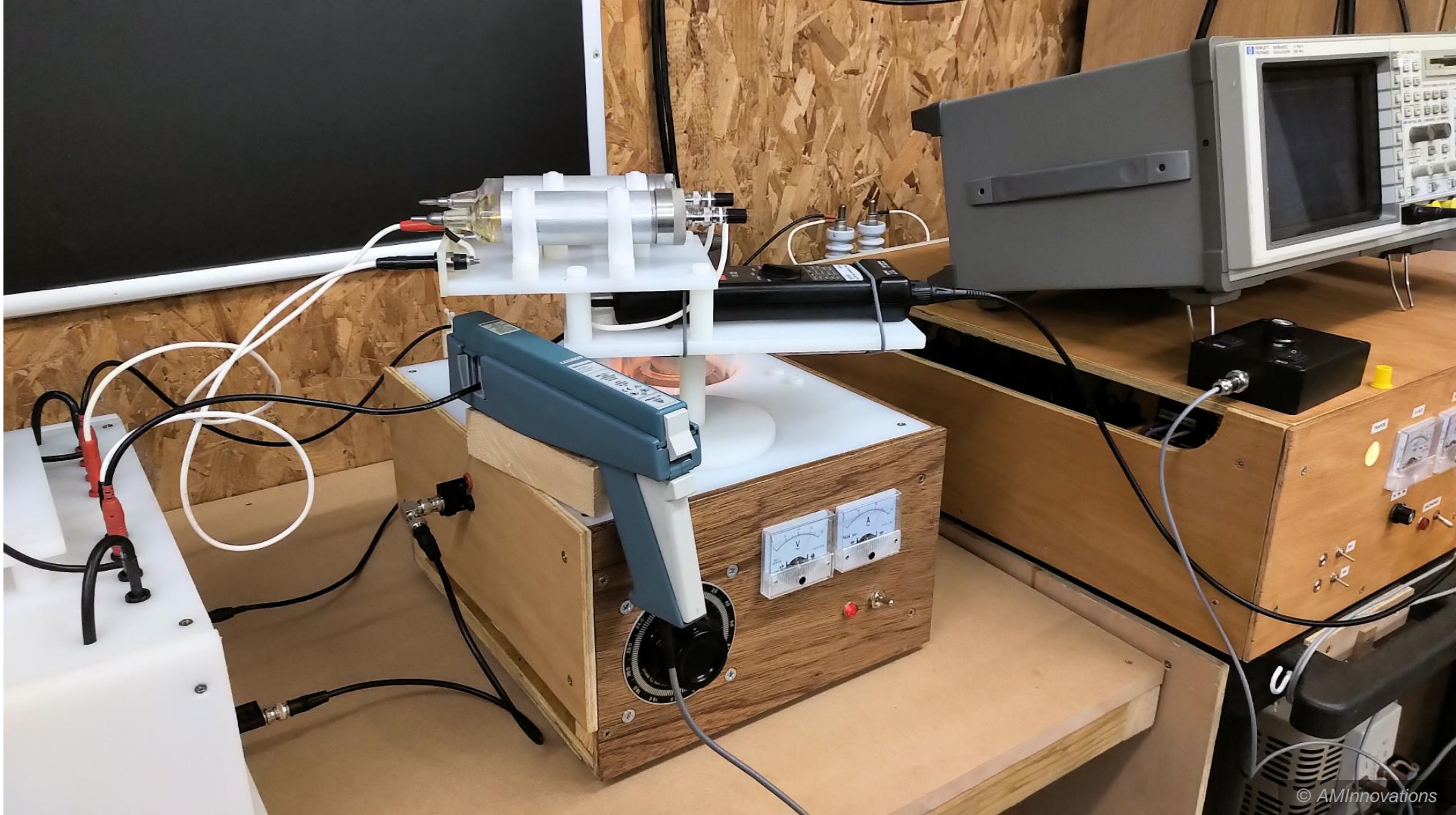
Extra High Voltage Differential Probe 80kV pk-pk, and Tektronix A6303 100A Current Probe
